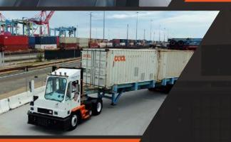
**HIGH LOAD CAPACITY** 90,000 lbs. GCWR 180,000 lbs. GCWR **SPEED** Up to 32 MPH Up to 32 MPH **LARGE BATTERY CAPACITY** 243 kWh
